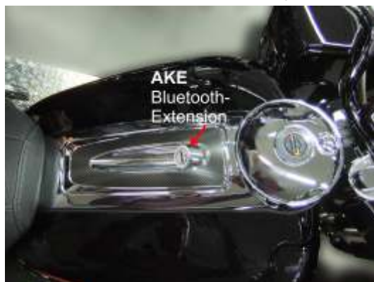
Fitting into the cover of the fuel tank instead of the helmet connection socket for the driver
