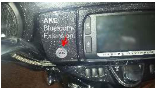
Fitting into the front panel instead of helmet connection socket of the audio system
