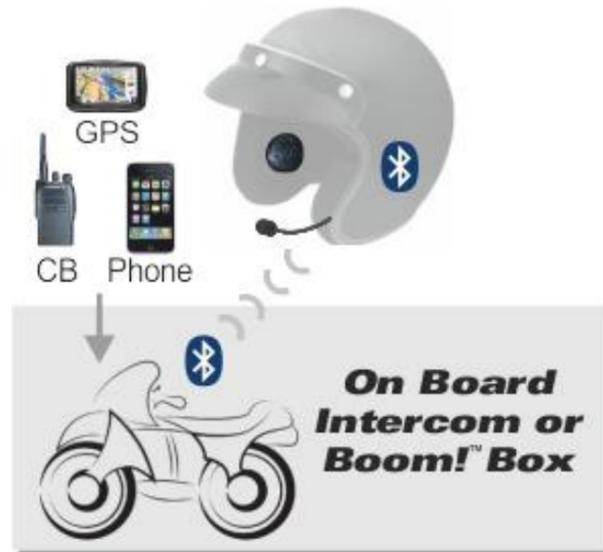
Bluetooth and cable from bike to helmet, stereo audio and intercom via board electronic
